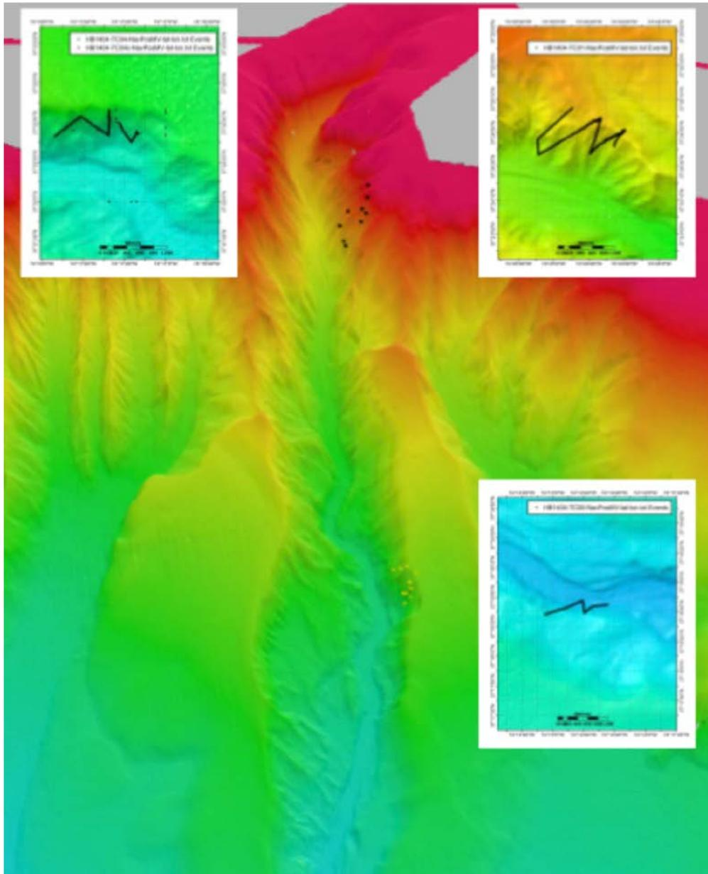
Bathymetric (topographic) map of the incised Washington Canyon (red = ~500 meters, green = ~2000 meters) insets show each of the TowCam surveys, with track line showing the area covered in the three tows conducted in 2014.
