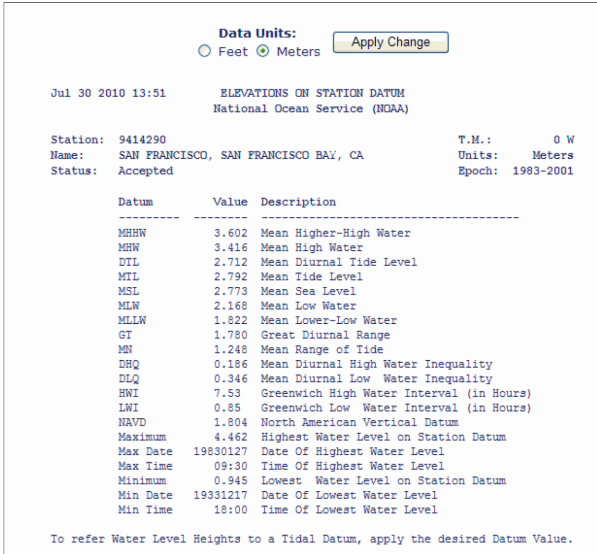
Figure 5. Accepted 1983-2001 NTDE datums for San Francisco. From http://tidesandcurrents.noaa.gov . NAVD refers to the North American Vertical Datum of 1988. Notice the differences in the values between the various datums.
